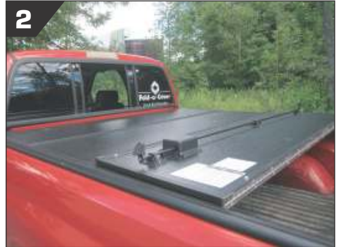
To insure proper operation of the center latch mechanism always open and fold the rear panel of the cover to its fully open position before starting any folding motion of the second or third panels.
