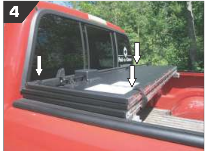
With the cover in the fully open and stacked position secure all three docking straps. It is important to secure the docking straps at all times when the cover is in the fully open position.
