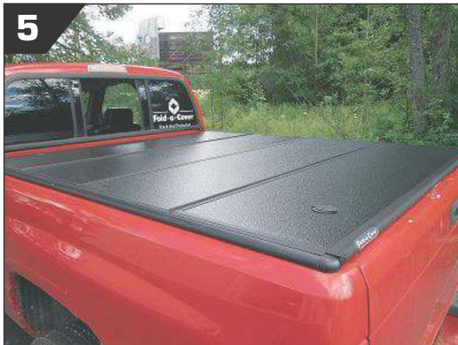
To close the cover, reverse these steps in the same order, making sure to close the rear panel last.
