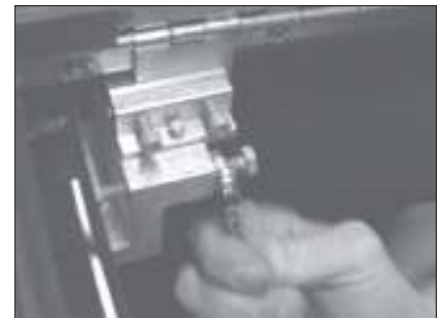
Pictured: Securing C-Clamp jam nut with 7/16" wrench.
