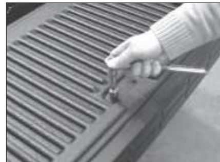
Pictured: Removing tailgate bolts.
