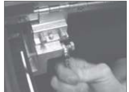
Pictured: Securing C-Clamp jam nut with 7/16" wrench.
