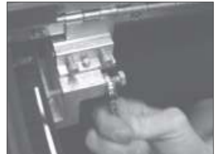
Pictured: Securing C-Clamp jam nut with 7/16" wrench.
