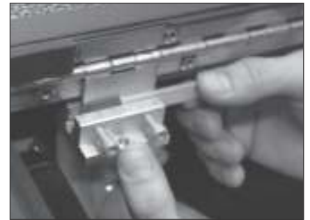
Pictured: Attaching Hinge Bracket to Cover.
