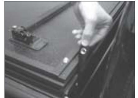
Pictured: Detaching snap restraint from cover.
