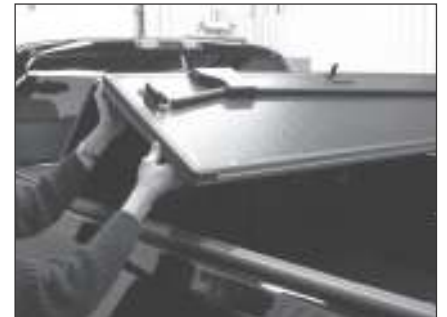
Pictured: Unfolding cover between wind seal rails.
