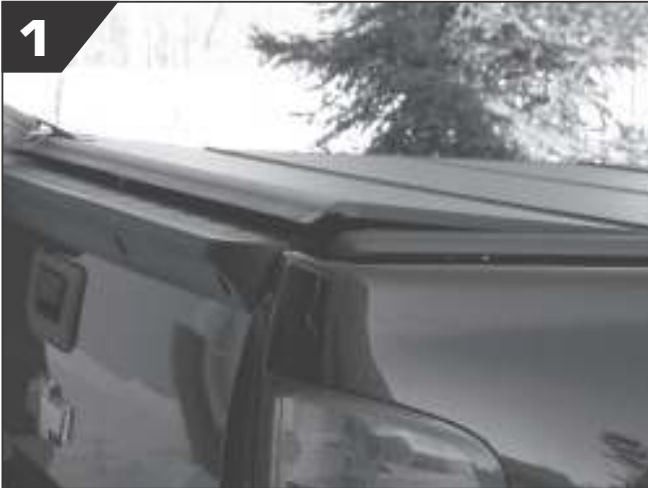
To open the cover lift the latch release handle and open the rear panel to the fully open position.
