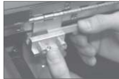
Pictured: Attaching Hinge Bracket to Cover.
