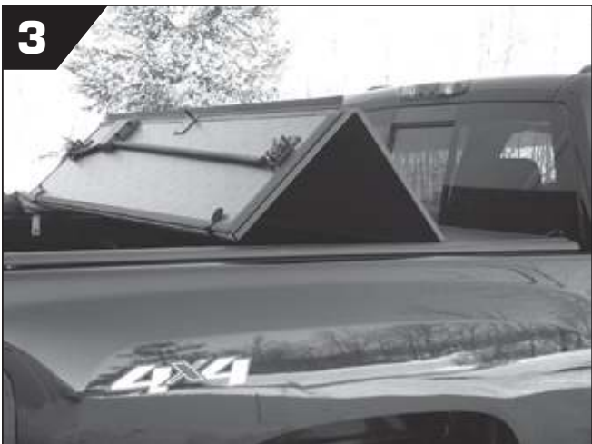
Continue the opening sequence by folding the second and third panel to the fully open position.
