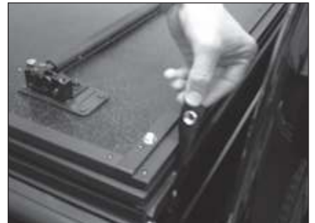
Pictured: Detaching snap restraint from cover.
