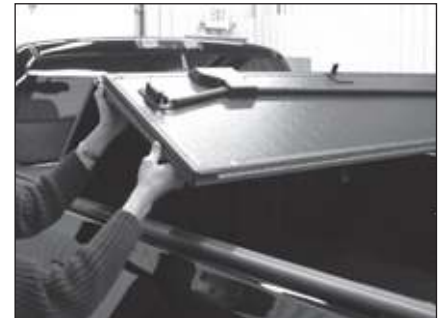
Pictured: Unfolding cover between wind seal rails.
