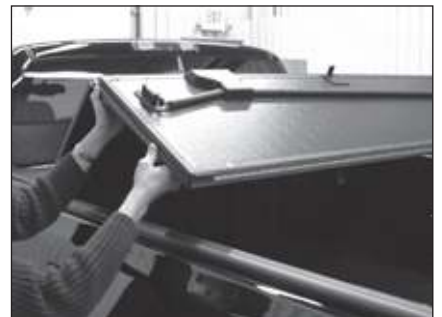
Pictured: Unfolding cover between wind seal rails.
