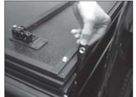
Pictured: Detaching snap restraint from cover.
