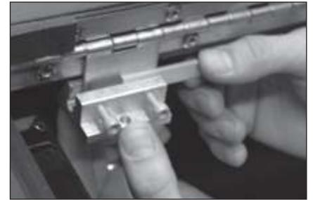
Pictured: Attaching Hinge Bracket to Cover.
