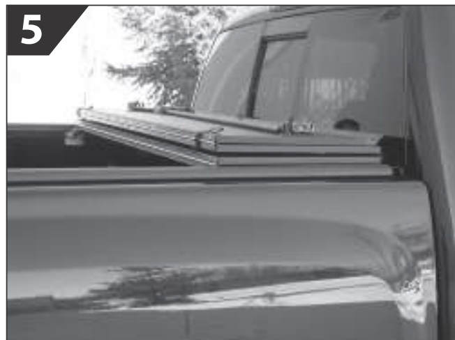
5 To close the cover, reverse these steps in the same order, making sure to close the rear panel last.
