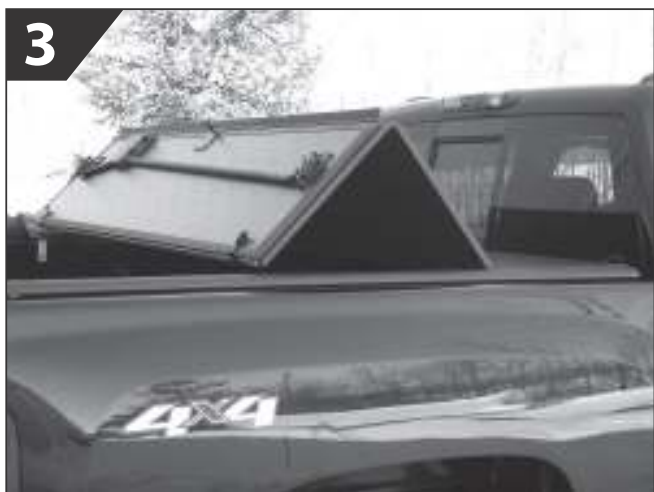
3 Continue the opening sequence by folding the second and third panel to the fully open position.
