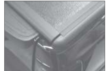
Pictured: Unfolding cover between wind seal rails.
