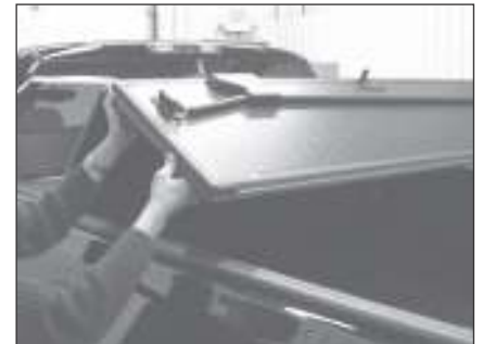
Pictured: Unfolding cover between wind seal rails.
