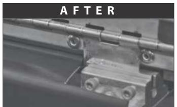
Tuck the bulb seal under the hinge as shown in the before/after imagaes. Start at each side and work to the center of the seal until the entire seal is under the hinge of the 2nd panel.
