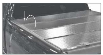
Close the front panel of the cover. It will be necessary to use a strong steady downward force and follow through to close this panel as air is trapped in the Caddy as the cover nears the closed position. If the cover does not close and latch with reasonable closing force it may be necessary to readjust the height of the striker bolts.
