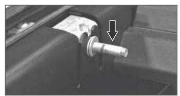
Reinstall the striker bolt and t-nut making sure the washers are in position to clamp the end panel of the Caddy as shown above. Adjust the height of the t-nut to the marks that were previously made. Using a 5/16" wrench tighten the striker bolt in place.
