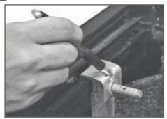
Using a pencil, mark the height position of the t-nut in the striker clamp assemblies as shown above. Using a 5/16" wrench, loosen the striker bolts and remove with the t-nuts. Set them aside for a later step.
