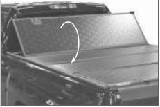
Fully open the forward panel (directly behind the cab) of the Fold-a-Cover® tonneau cover. Make sure the key is not in the lock and that the lock cover is closed to prevent damage.
