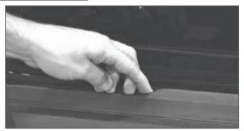
Fold the front seal over the edge of the factory bed liner or against the bulkhead as shown above and to the right.
